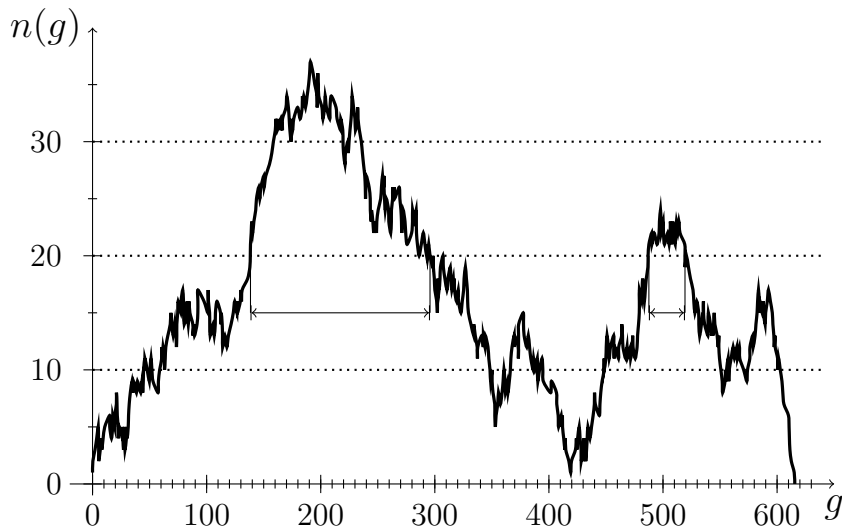
FIGURE 1. Example of thresholding of a time series. An event begins when the signal exceeds the threshold (dotted lines, h = 10, 20, 30 ) and ends as soon as the signal falls below the threshold. Increasing levels of the threshold lead (non-monotonically) to different numbers of events and, provided the signal eventually ends, monotonically smaller total event durations. The main focus of this paper is on the statistics of the individual event durations, as exemplified by the two intervals for the intermediate threshold.
