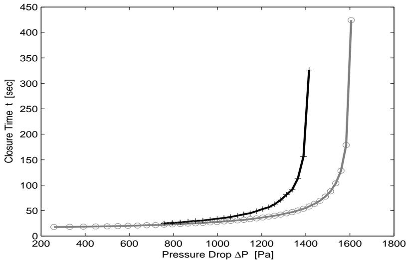
FIGURE 3. The closure time against the imposed pressure drop across the channel for blood when  $T_0 = 9.3^\circ\text{C}$ ,  $T_f = -0.3^\circ\text{C}$  and  $T_w = -3.27^\circ\text{C}$ . Circles points are those for the non-Newtonian case, whilst the cross points correspond to the equivalent Newtonian case. The lines are for guidance.
