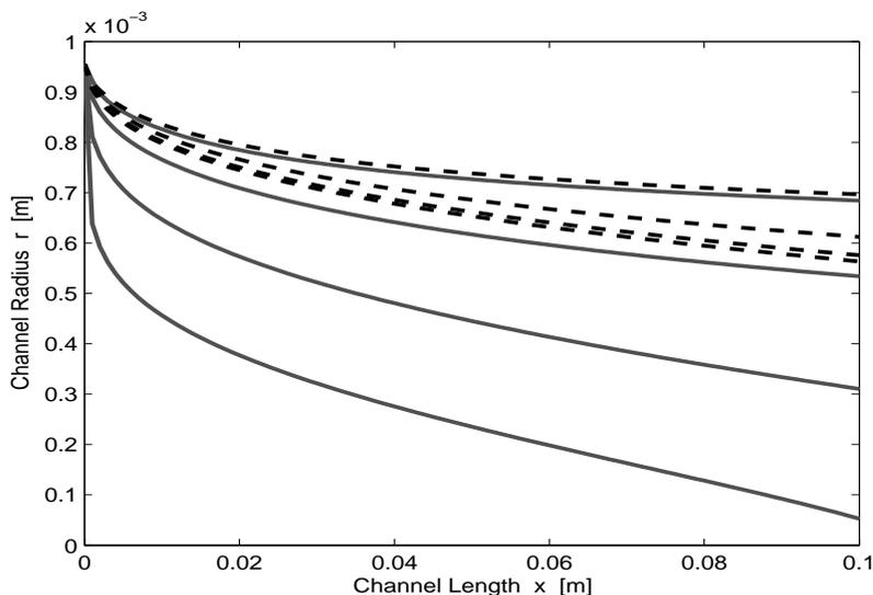
FIGURE 4. The position of the solidification fronts for PEO at times  $t = 57.3, 118.1, 319.0, 384.4$ s. The solid lines represent the non-Newtonian model, the dashed lines are the equivalent Newtonian case.
