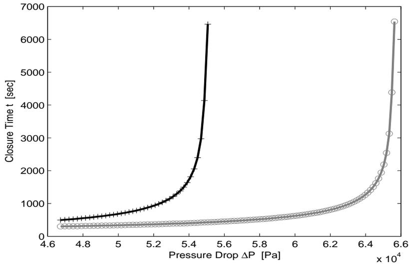
FIGURE 5. The closure time against the imposed pressure drop across the channel for Polyethylene oxide when  $T_0 = 73^\circ\text{C}$ ,  $T_f = 63^\circ\text{C}$  and  $T_w = 59.9^\circ\text{C}$ . The circle points correspond to the non-Newtonian case whilst the crosses are those for the Newtonian and the lines are for guidance.
