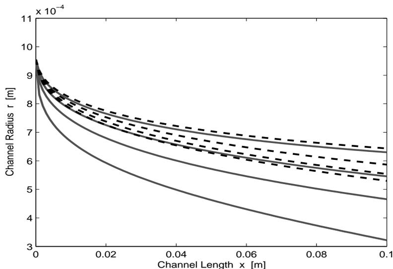
FIGURE 2. The position of the solidification fronts for blood at times  $t = 9.9, 20.5, 31.1, 41.7$ s. The solid lines represent the non-Newtonian model, the dashed lines are the equivalent Newtonian case.
